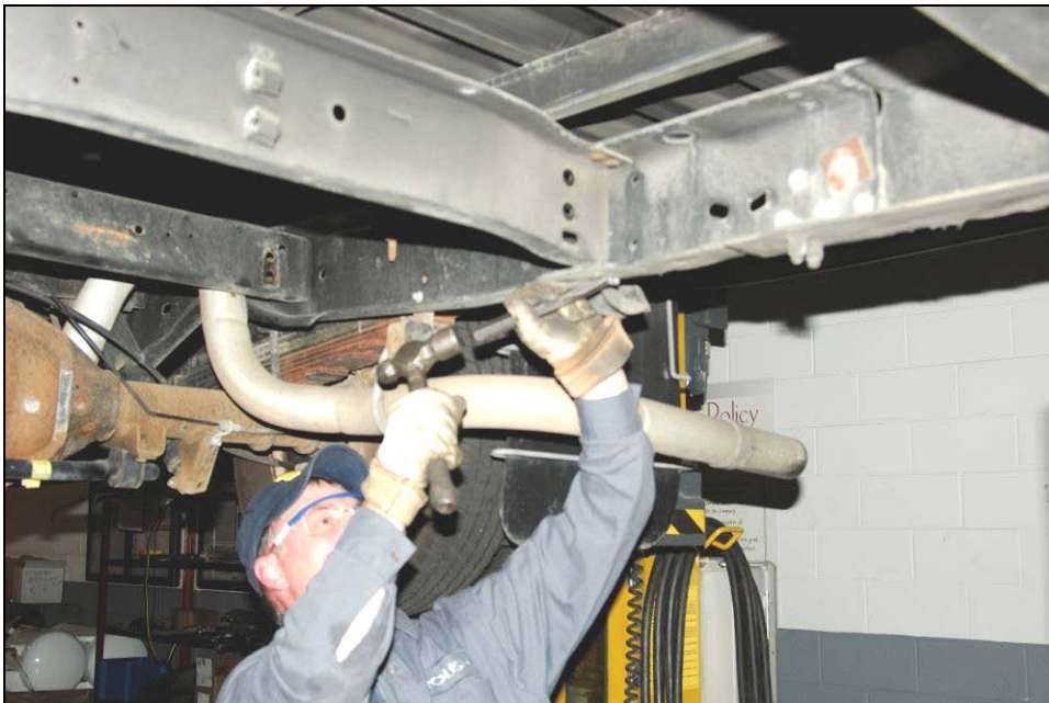
Chiseling Lower Rear Crossmember Rivet
