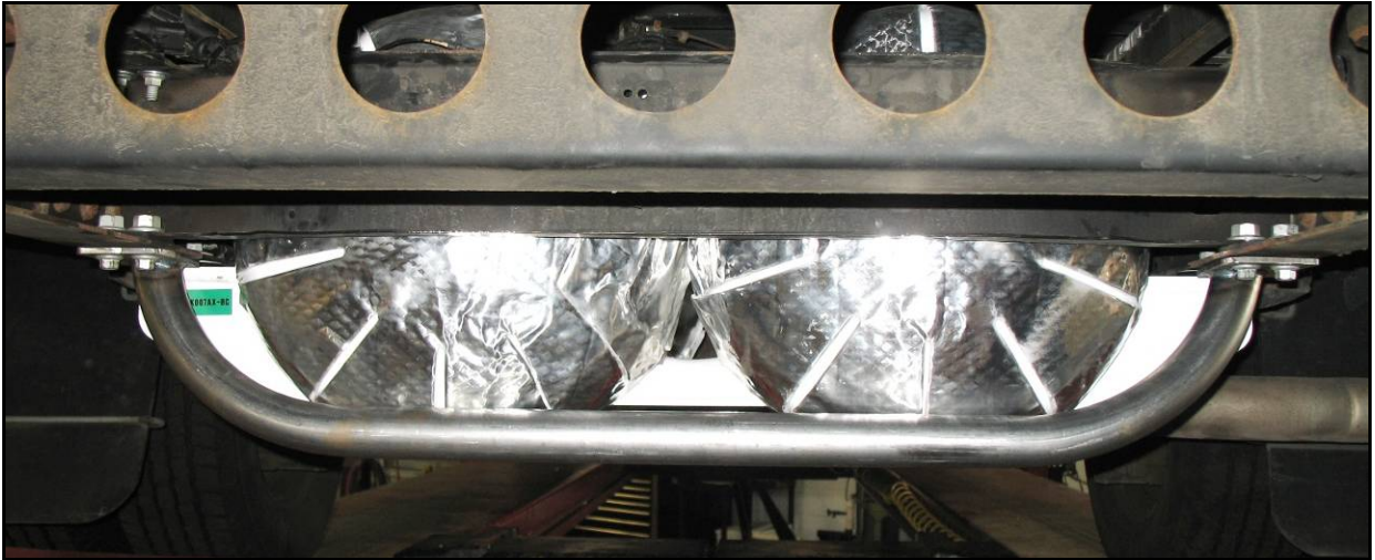
Relocated Rear Crossmember and Fuel Tank Guard Installed
