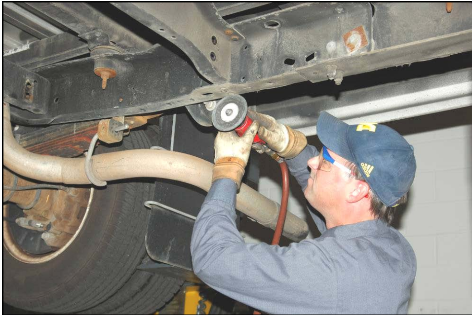
Cutting Lower Rear Crossmember Rivet
