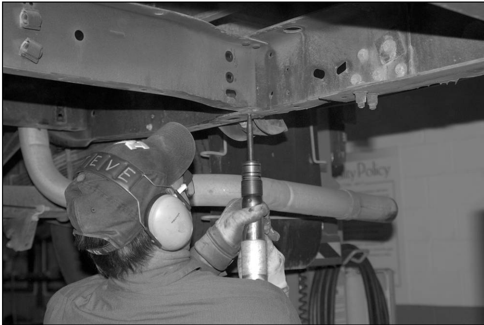
Punching Out Rear Crossmember Rivet
