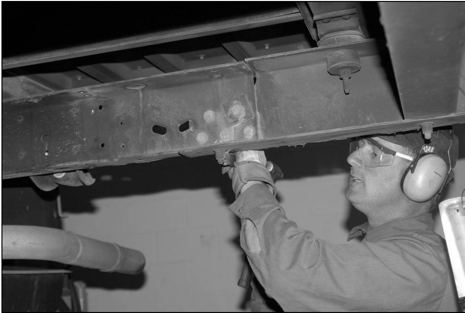
Separating Lower HUCK™ Collar from Pin
