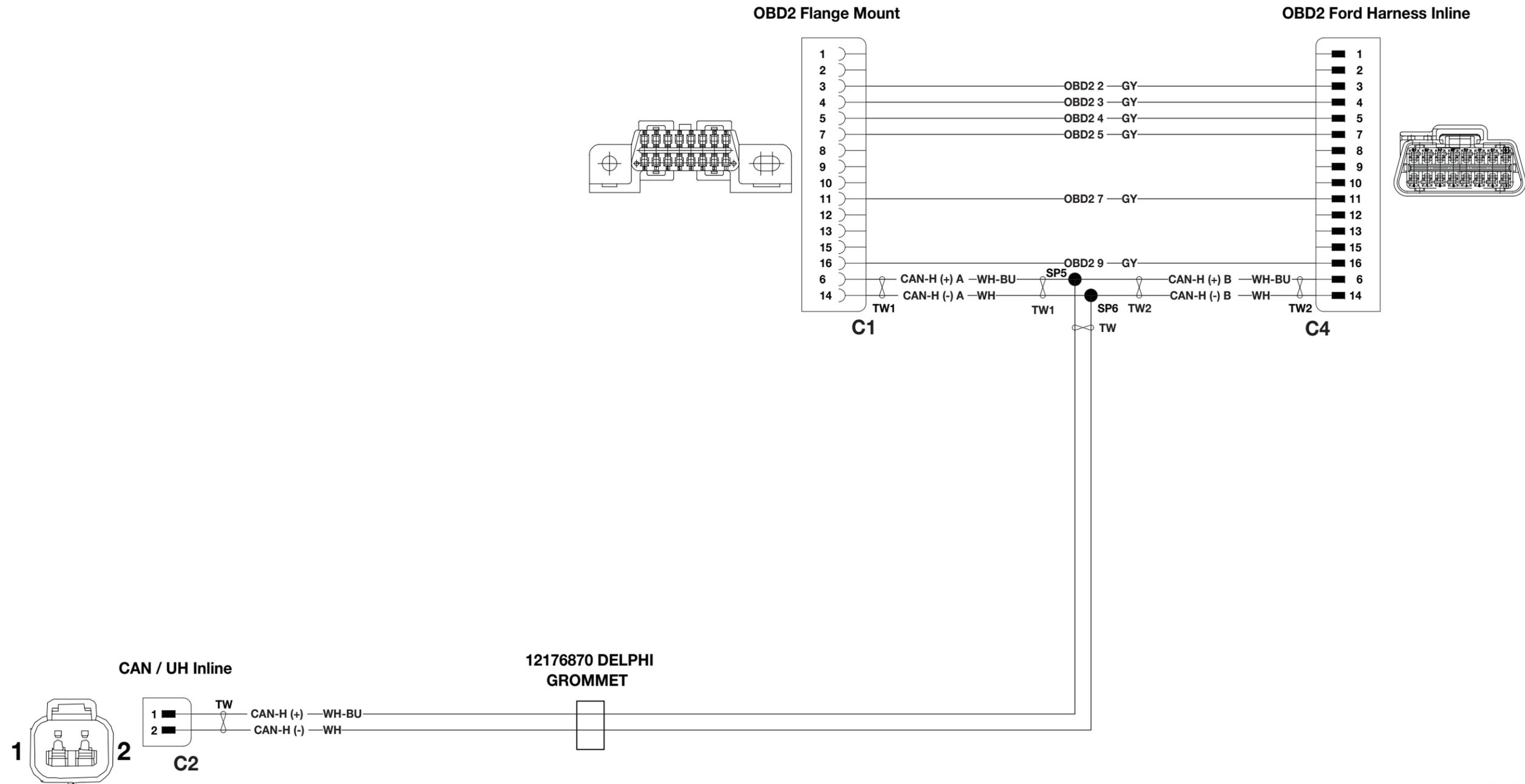
**E-450 Electrical Schematic — Tank Harness**
