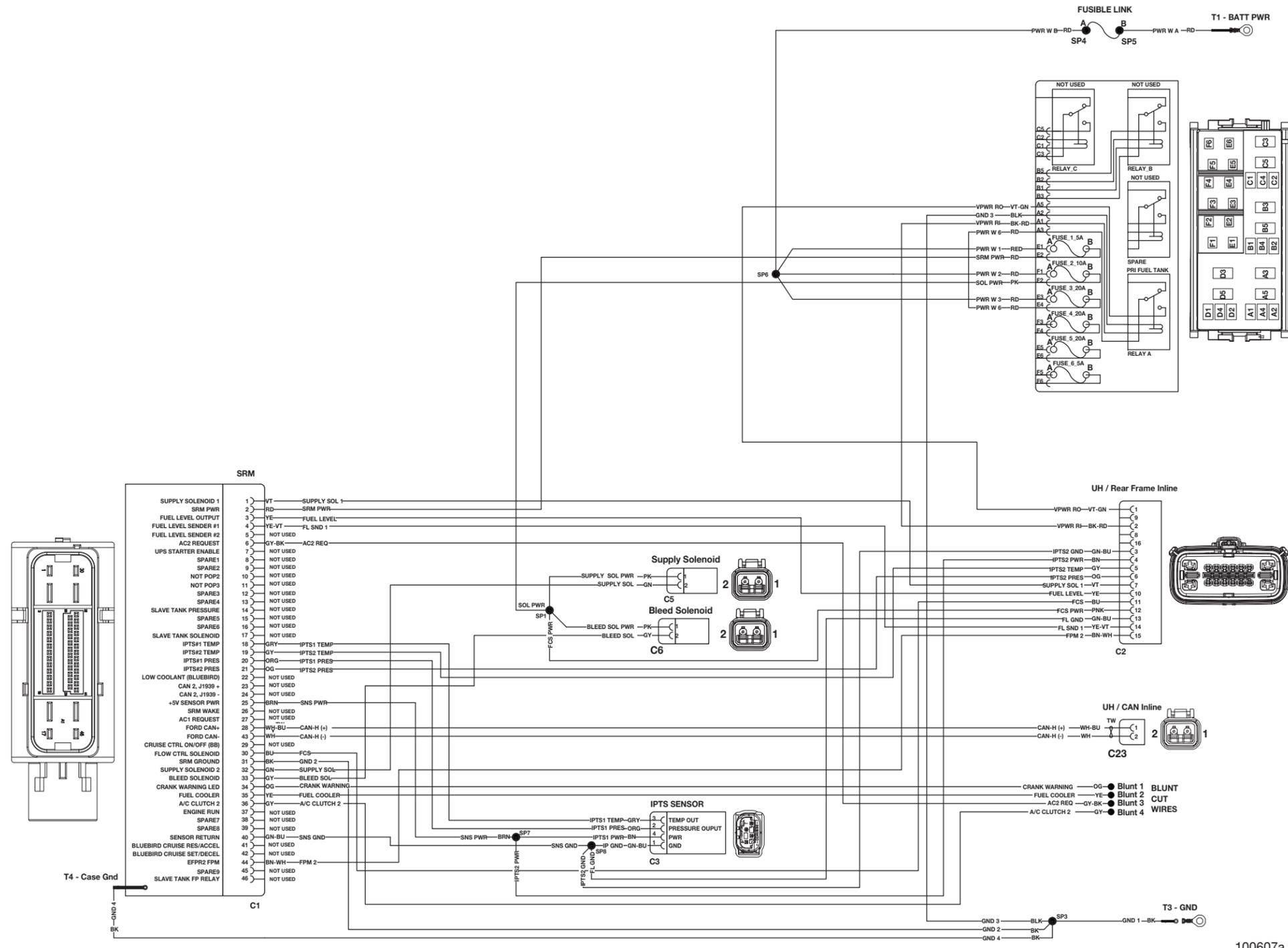
**E-450 Electrical Schematic — CAN Bus Harness**
