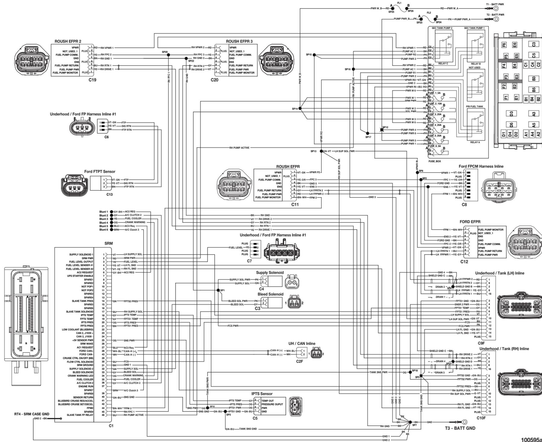
**F-650 F-750 Electrical Schematic — CAN Bus Harness**
