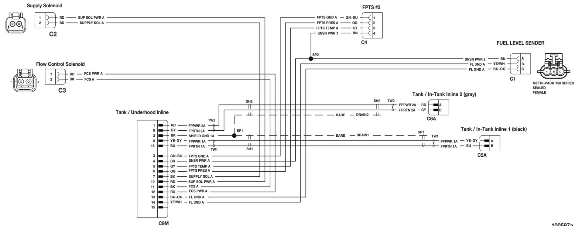
**F-650 F-750 Electrical Schematic — Right Tank Harness**
