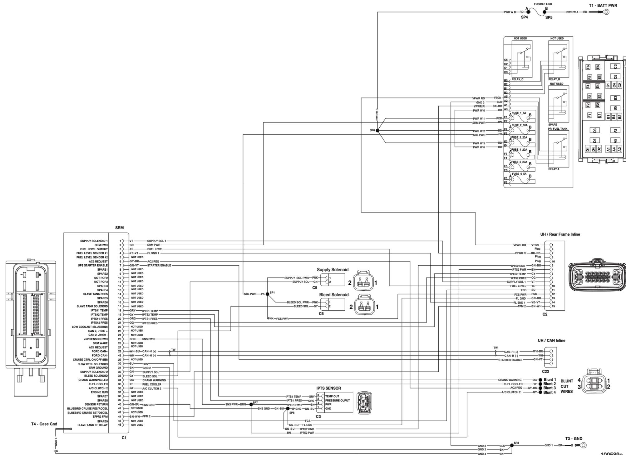
**F-59 F-450 F-550 Electrical Schematic — CAN Bus Harness**
