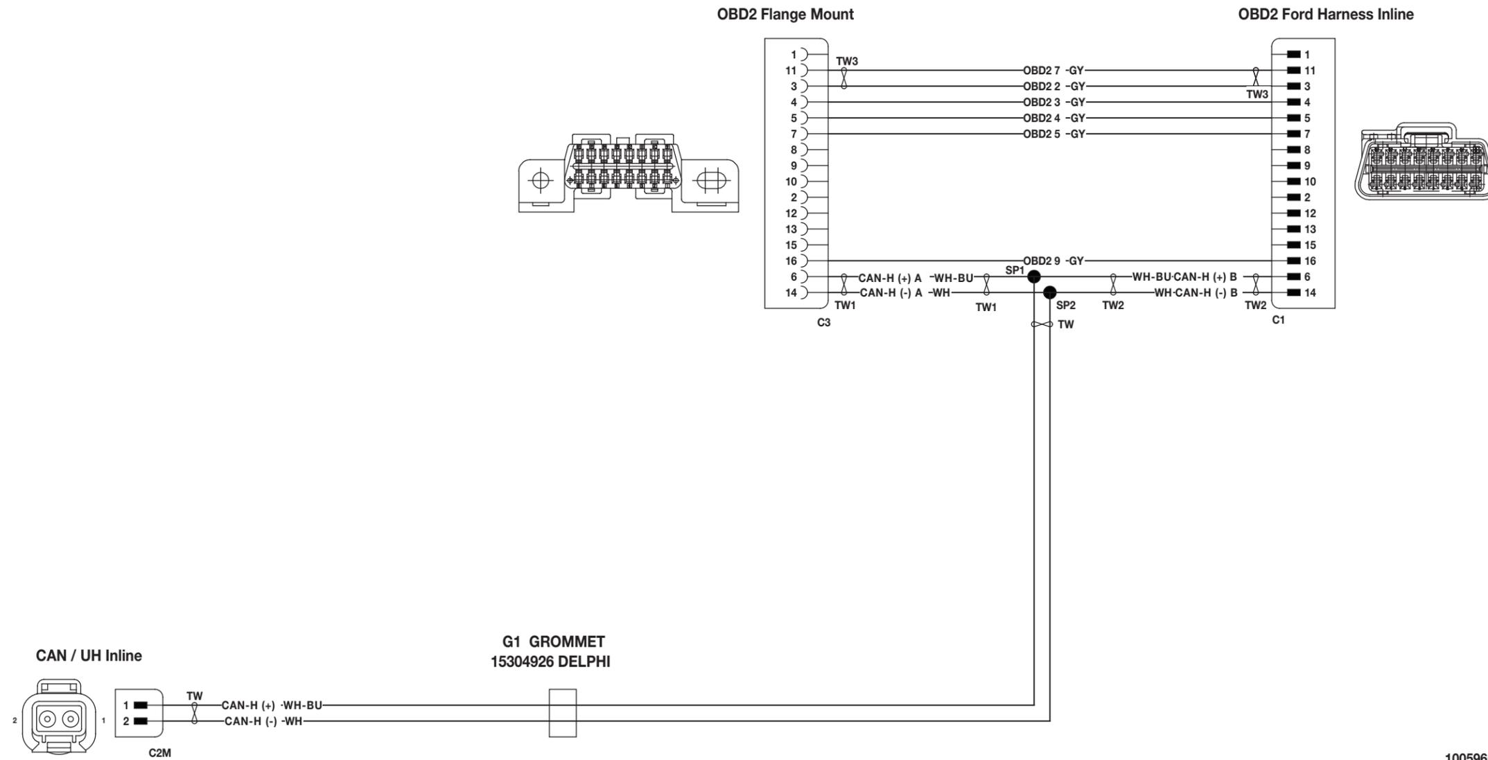
**F-650 F-750 Electrical Schematic — Left Tank Harness**
