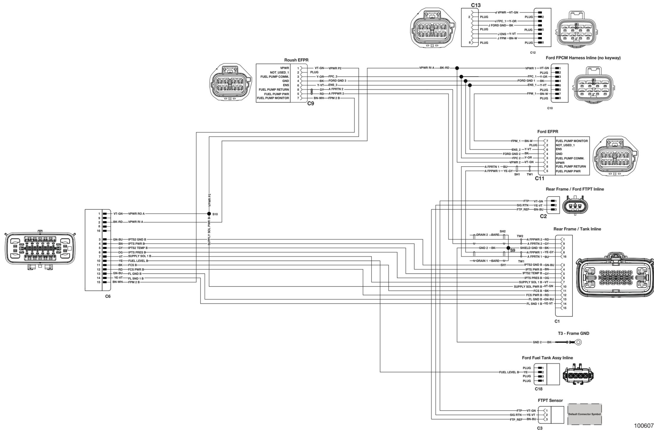
**E-450 Electrical Schematic — Rear Frame Harness**
