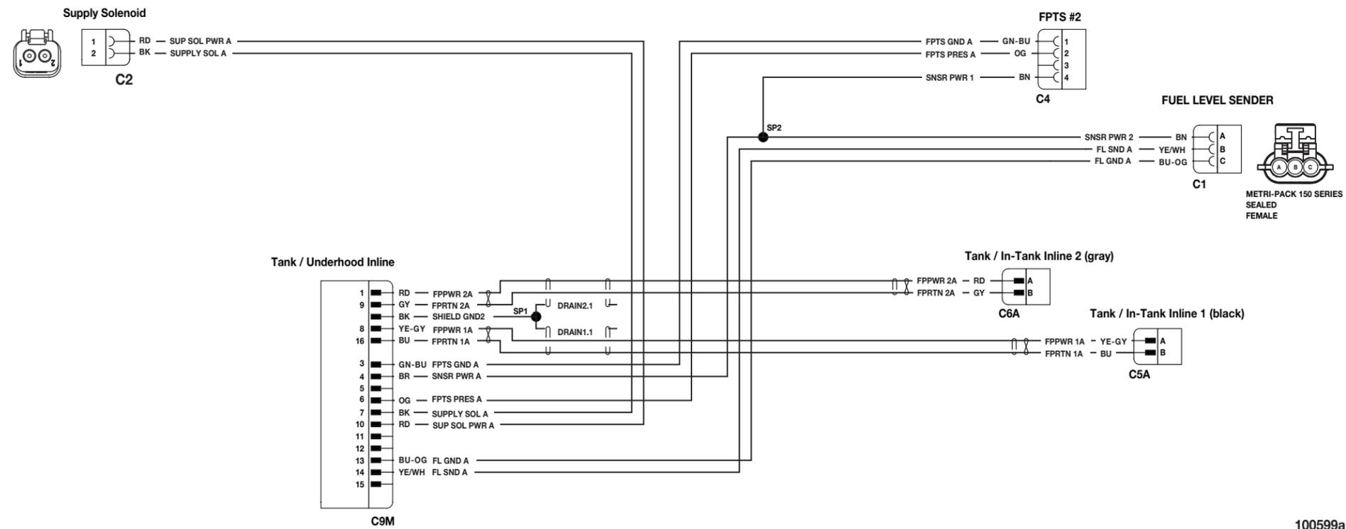
**F-650 F-750 Electrical Schematic — Transfer Overlay Harness**
