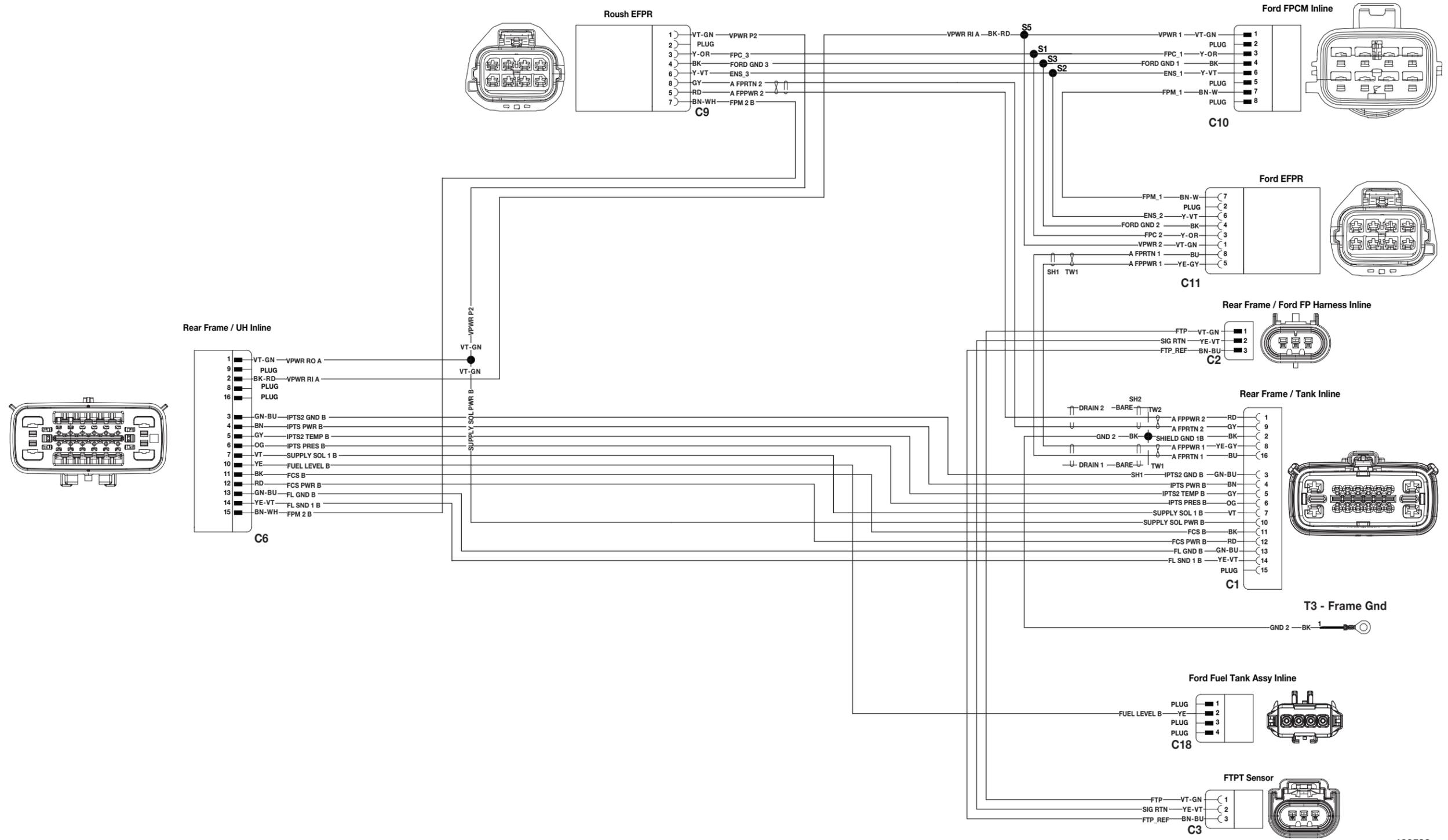
**F-59 F-450 F-550 Electrical Schematic — Tank Harness**
