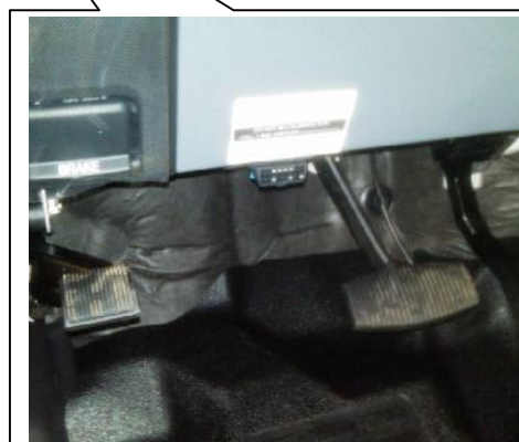
PCM Tamper Warning Label (R07100008-A) on knee bolster above OBDII diagnostic port
