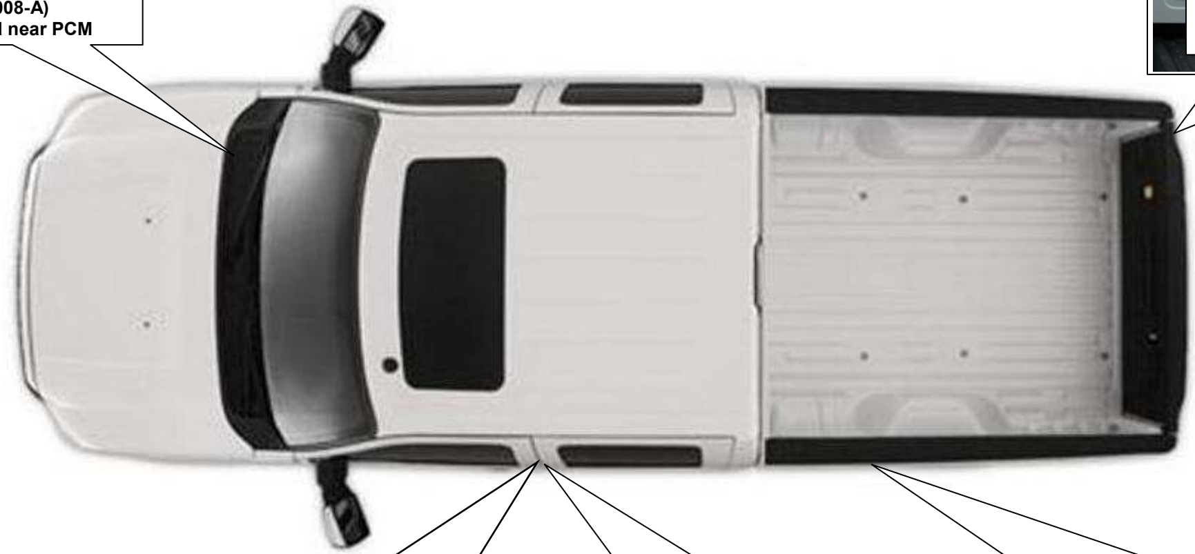
Overfill Protection Device Label (P11BB-01C200-B) at mid-door HD5 Propane Label (P07L3-9A095-A) at top 350 PSI Working Pressure Label (P07L3-9A095-I) at bottom center left
