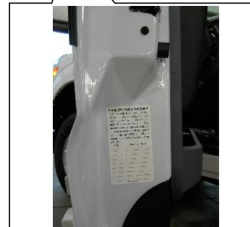
Bleeder Valve Inspection Label (P07L3-9A095-C) to end of driver door
