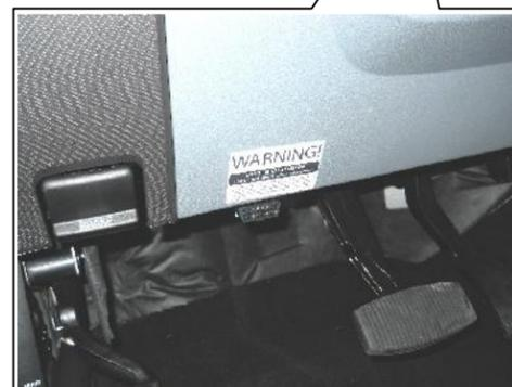
PCM Tamper Warning Label (R07100008-10-A) on knee bolster above OBDII diagnostic port
