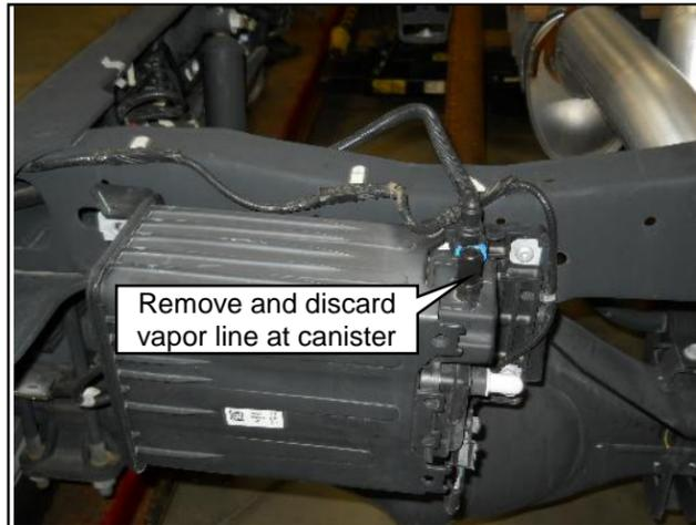
Figure 3.4 — OEM Midship Tank: Canister Location
