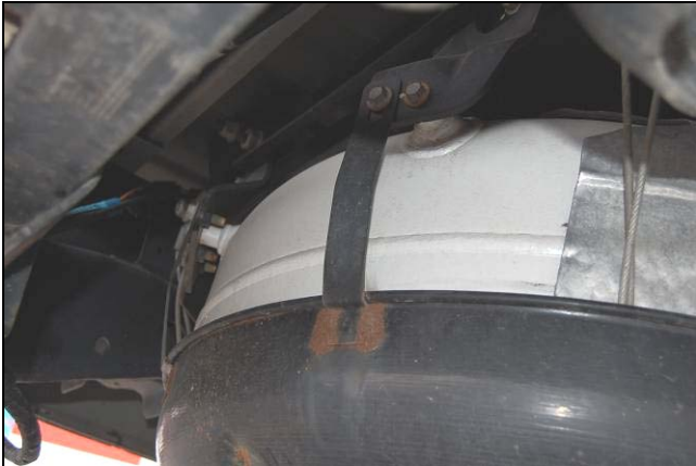
Figure 64 — Fuel Tank Safety Tub and Cables
