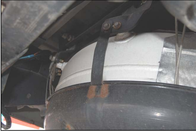
Figure 56 — Fuel Tank Safety Tub and Cables
