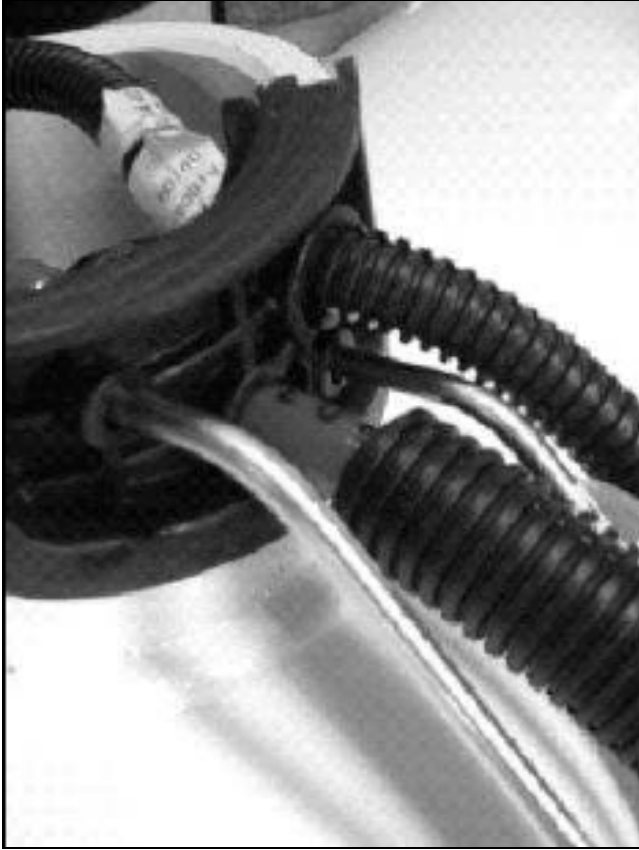
Figure 68 — Fuel Lines, Wiring and Convolute Tubing
