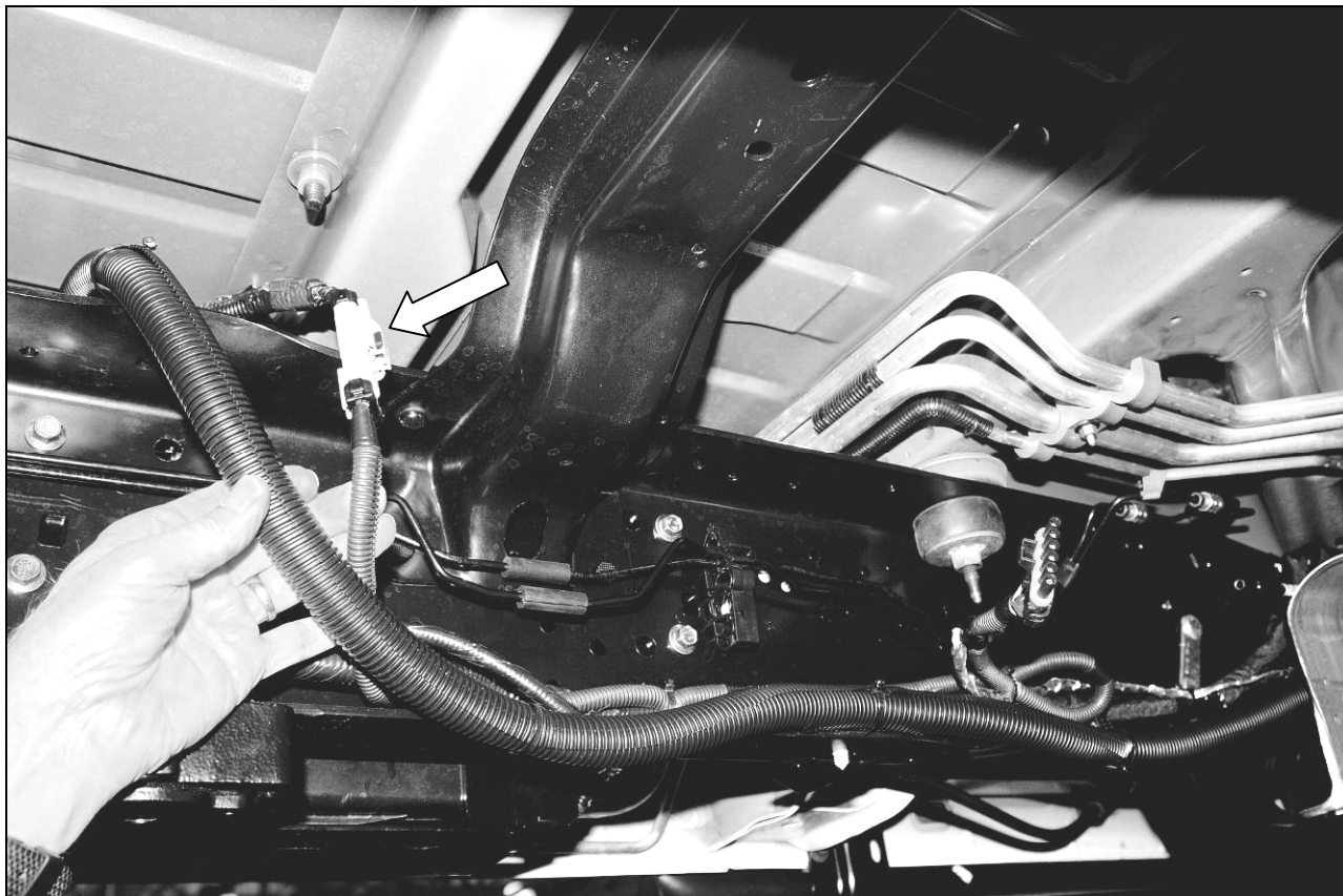
Figure 19 — ROUSH CleanTech-to-Ford 4-Pin Harness Connector (Typical)
