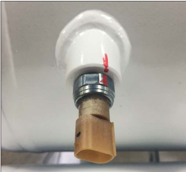
Figure 19 – Tank Pressure Temperature Sensor
