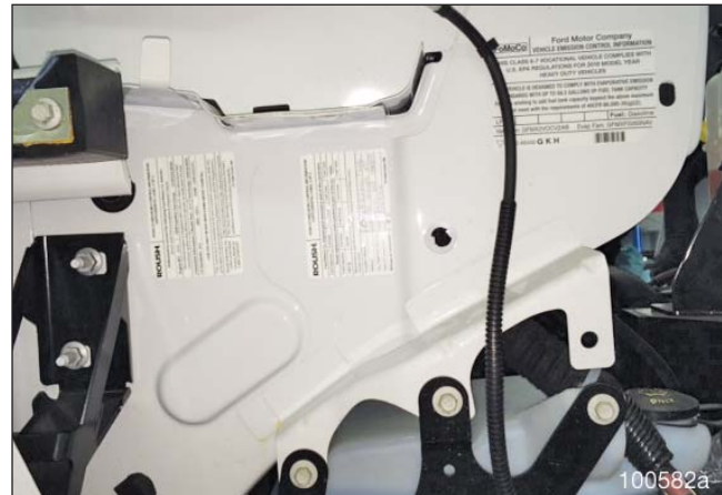
Figure 7 – F-650/750 VECI Label Body Location – Passenger Side
