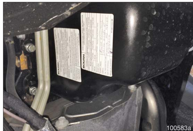
Figure 8 – F-650/750, F-59 VECI Label Oil Pan Location – Passenger Side Oil Pan
