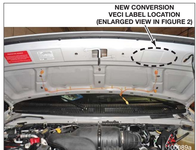
Figure 3 – VECI Label Location (Typical Placement)
