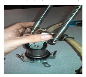
3. Install the three Allen bolts into the bracket and torque them to 10Nm.
