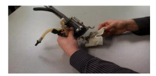
2. Remove the connector from the side of the top mounting bracket using trim tool.
