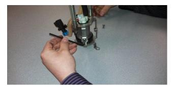
4. Remove the pump motor from the bracket for replacement.
