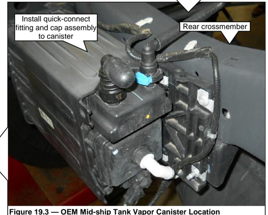
Figure 19.3 — OEM Mid-ship Tank Vapor Canister Location
