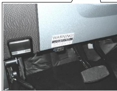
PCM Tamper Warning Label (R07100008-10-A) on knee bolster above OBDII diagnostic port
