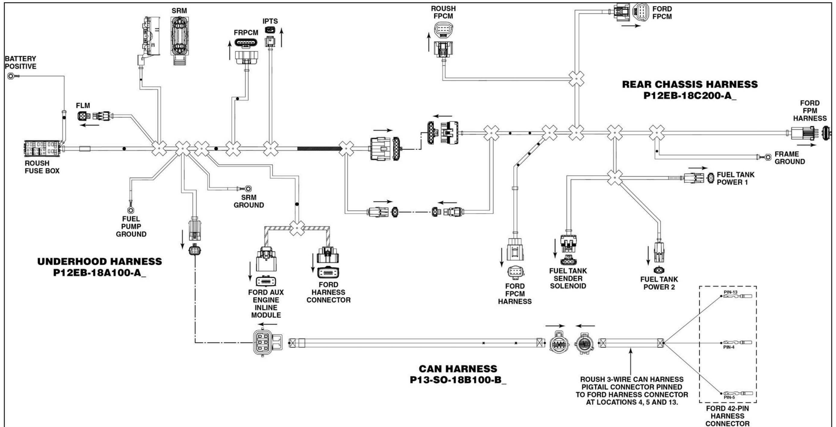
WIRING HARNESS CONNECTOR LAYOUT — F-450/F-550 CHASSIS CAB G.A.S. CONVERSION
