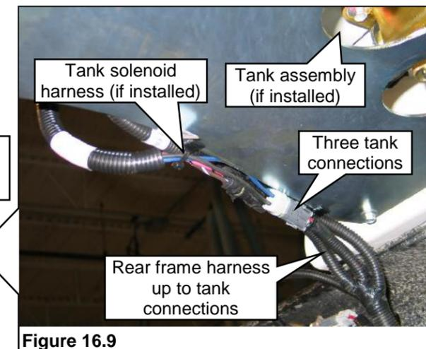
**EFPR Location Originally Equipped with Aft-axle Gasoline Tank**
