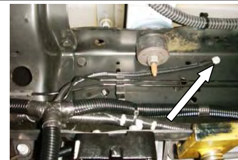
Rear frame harness (P11GD18C200-A) ground — use M6 x 1.0 x 16 bolt (W500213-S437) and nut (90591A151). Tighten to 8–12 Nm.
